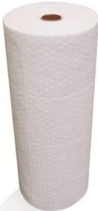
Dimpled meltblown polypropylene sorbents are most commonly used to skim oil off of water. Their fibrous texture draws hydrocarbon-based fluids into the center of the pads and/or rolls while repelling water.
